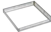
**DrainGuard** – An all too common sight around a roof drain is the accumulation of leaves, pine needles and other debris that can restrict water flow, potentially causing a dangerous situation. A simple solution is to install a 4-in. high by 4-ft. x 4-ft. square (or 3-ft. x 3-ft.) perforated DrainGuard around the drain holding back debris but allowing water to pass to the drain.
