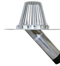
**Custom Drains** – Though most new and retrofit roof drain installations conform to standard industry practices, there are the occasions when an unusual condition occurs at a drain location. In such instances, the standard drain may need to be modified or custom designed to fit the particular site conditions. OMG Roofing Products recognizes this need and can accommodate most custom requests. Please contact OMG at 800-633-3800 to review the application.
