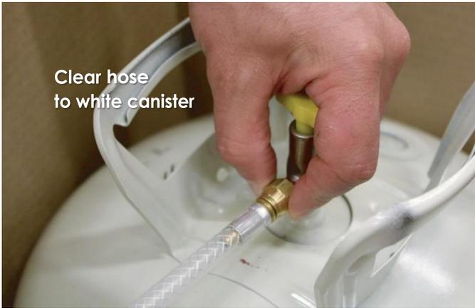
**STEP 6.** Tighten both fittings with the 9/16-in. wrench (provided) by turning an additional 1/6 turn until firmly attached. **DO NOT OVER-TIGHTEN!** Close lid of each box to protect from sun, wind and dirt.
