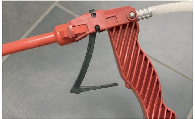
**STEP 9.** It is recommended to verify the canisters are properly reacting and curing before using. Spray onto scrap piece of substrate (iso, deck or coverboard) and monitor the reaction.
