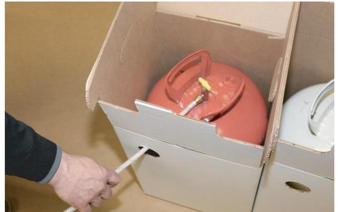
**STEP 4.** Attach swivel fitting on red striped hose, finger tight, to the valve outlet on top of the red cylinder.
